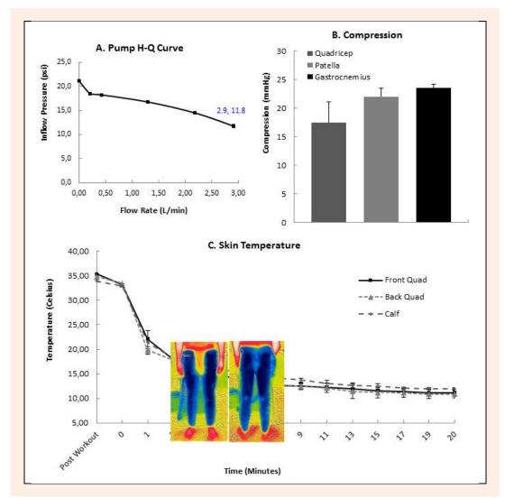
Figure 3. Equipment study on the different mechanical and engineering characteristics of the Cryocompression (CRC) System (Aquilo Sports, Louisville, KY, USA)
